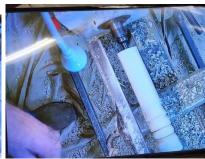
Jim Mencum then demostated some techniques with the Skew. Jim cautioned about catches and demostated how they can occur. Through no fault of his own Jim demostrated how ineffective and dangerous a dull tool (Skew) can be. Jim emphasized the need to keep your tools sharp.
