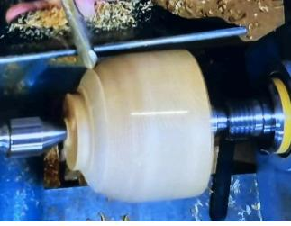
After checking alignment he reverted to a bowl gouge and formed a tenon.
