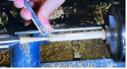
Using a 4 jaw self centering chuck and a ring center on the tailstock. 3/8 skew.
