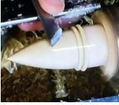
He showed us the Axminster O'Donnel jaws and mounted more softwood in it. Tool rest was high again. He moved to a smaller ¾ skew and shaped the piece to a sharp point. He then cut a groove with the short point and pushed the fibers back. The heal forms them. He repeated again and again.
