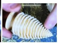
Finally he used the Russian Skew to part it off. It is finished with an airbrushed color.
