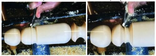
He turned down the shoulder and started the taper of the leg with a spindle gouge.
