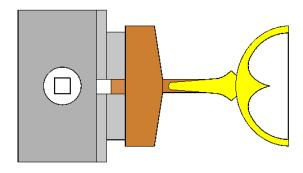
Remove excess wood, finish turning the stim, and carefully part it off.
