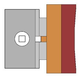
Turn a slight concave in the bottom. Leave a narrow flat on the outside edge of blank.
