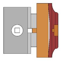
Drill a shallow %" diameter mortis for the golf ball seat (test ball for fit), and a smaller mortis for the tee.
