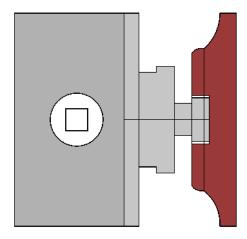
If you chuck jaws are not small enough, you can drill the glue block, turn a small plug to insert into the hole to use for alignment of the base. Attach base to glue block and finish base.
