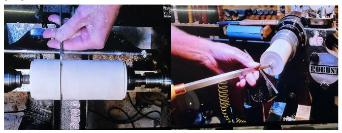
Carl turned tenons at both ends and then parted off the bottom and top. He took the bottom and chucked it up in his EasyWood chuck. He then cut off the nib
