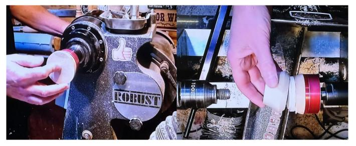
Carl has a piece of scrap permanently mounted on the Joyner off-center jig. He then attaches the scrap intended for the applique to it with double stick padded tape. The applique is then sized for the recess in the top,
