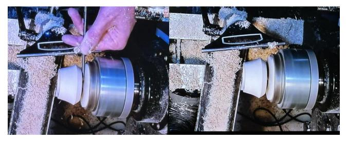
He then used the cavity of the top to mount on the EasyWood chuck with the expanding jaws. He was then able to form a recess for the applique. The rings are then attached with 5 minute epoxy.
