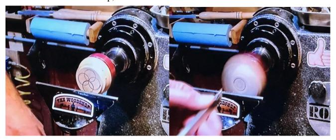
The pattern is tested in all four positions with a pencil which also establishes the design and a pattern. When all checks out a cutting tool is then used to cut the design.
