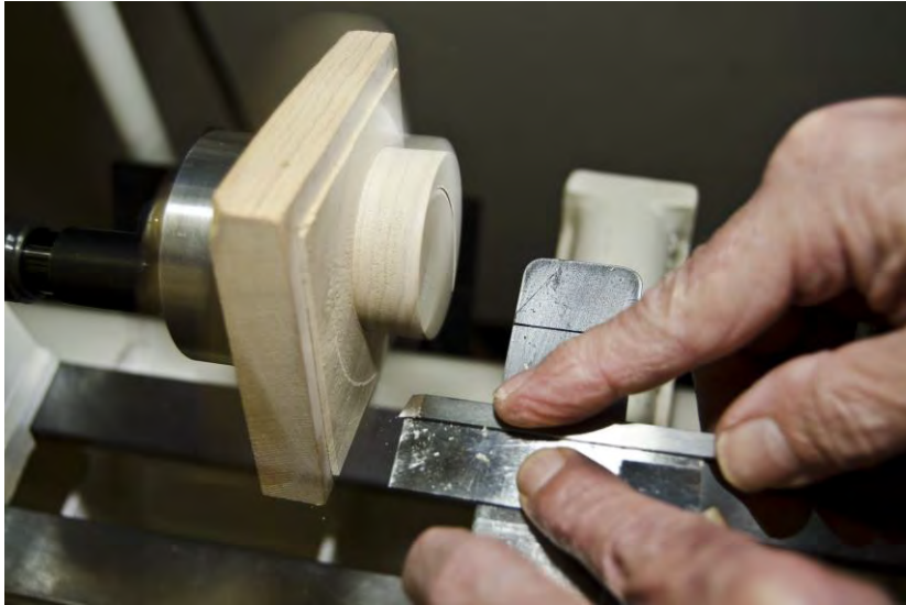
Figure 11 – Using a small square as a tool guide to make a shallow cut for a design element at a precise distance from the turning axis
