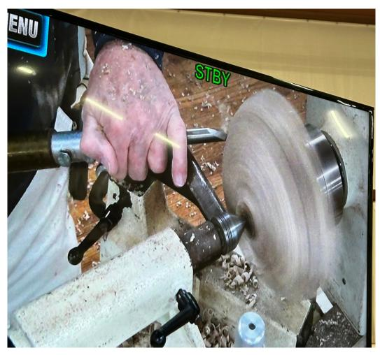
Bore a hole in the open bowl side of the work.
