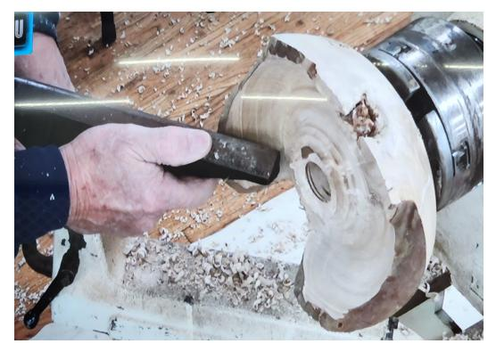
Ralph's discussed mounting the blank - center of blank vs center of mass - either is possible, with consideration of symmetric final appearance and dealing with the dynamics of an off weighted blank.
