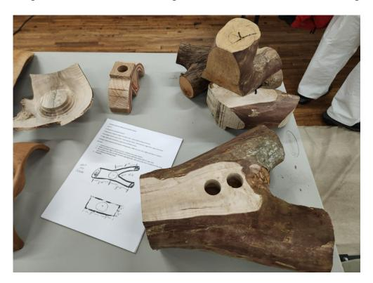
He emphasized the need to always work between centers. He generally uses a spigot chuck but said that you can use a spur drive if you bore a hole to receive it. He emphasized that the pieces are frequently out of balance and must be well secured for safety. He also reminded everyone to use a face shield and eye protection at a minimum because pieces may well come flying off. Ralph has a combined helmet, air source and face shield - the 3M Airstream.
