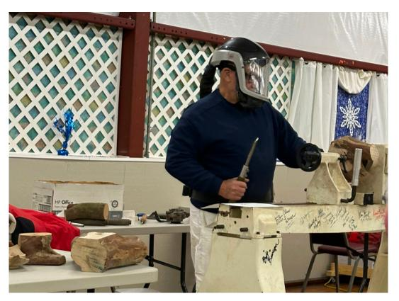
He advocated starting at a very low RPM until balance is achieved. Make sure that the tool rest is dogged down as you begin. Turn the assembly by hand before starting to make sure its clear.
