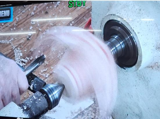
After initial mounting, goal is to shape the bottom and to form a tenon/spigot so that blank can be reversed into a spiral chuck for shaping/hollowing of inside and the wings. Back up chuck mounting with use of tailstock as long as possible for safety. Turn topside of wings same fashion as bottom.
