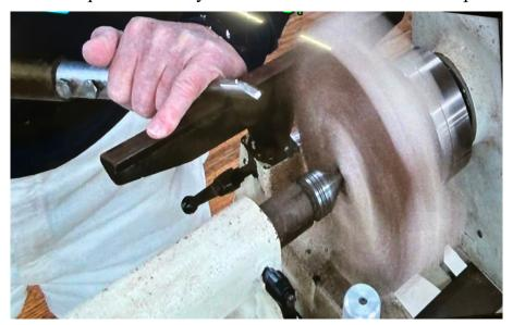
Ralph reminded us to turn pieces as close as possible to final finish because of the difficulty inherent in sanding this kind of work.
