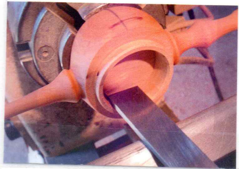
Step 11. Hollow inside diameter with bowl gouge or scraper and square insides with skew chisel. Sand surfaces.
