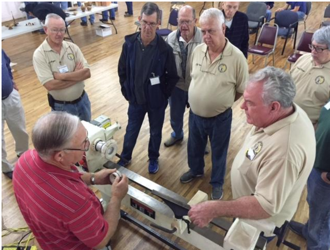
Earl Rennie explaining use of Cole jaws and Longworth chucks
