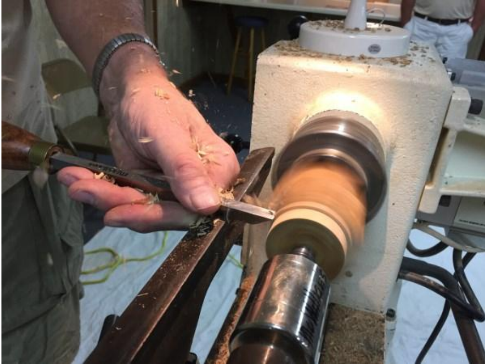
Rounding stock using bedan and Niles stopper chuck held in spiral chuck
