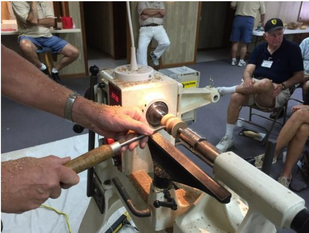
Shaping stopper with a spindle gouge, using pin chuck in headstock (with drawbore). Keeping stock between centers is big safety measure.
